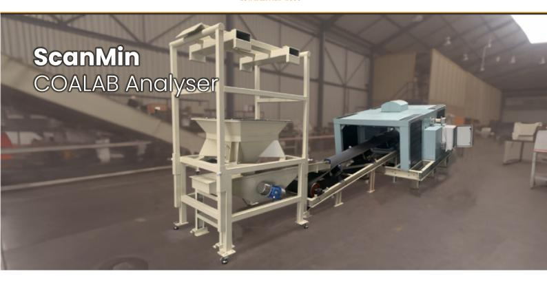
ScanMin Africa have developed a rapid bulk sample elemental analyser using our well-established Neutron Inelastic Scatter and Thermal Neutron Capture techniques.
