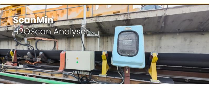
The H2OSCAN On-Belt Moisture Measurement System now allows the accurate measurement of moisture in real-time. This ready availability of moisture information allows proactive process control actions. The information can be used in several ways including:
