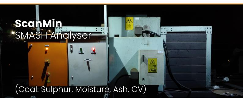
The ScanMin SMASH™ is a Prompt Gamma Neutron Activation Analysis (PGNAA) Elemental Analyser. The analyser uses a high-energy Am241Be radionuclide neutron source, which irradiates ALL the material on the belt as result of the temporary excitation of the atoms in the material This provide opportunity to measure two physical reactions:
