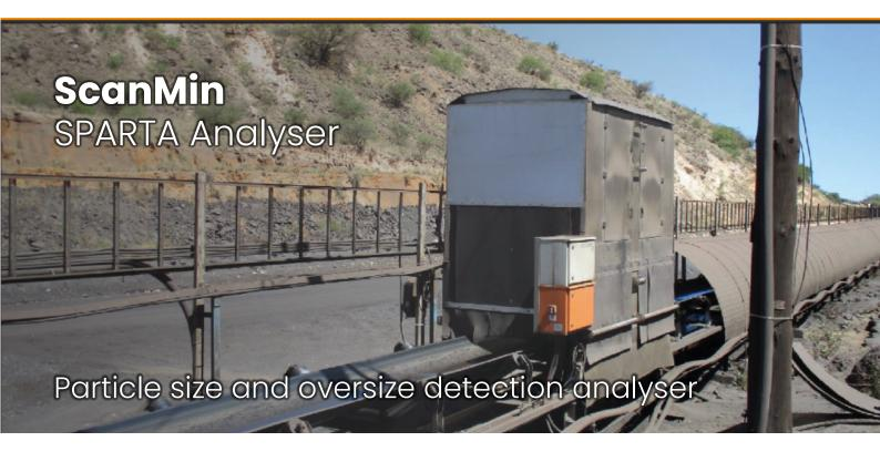
The ScanMin particle size analyser provides real-time automated analysis of particle size distribution on a conveyor belt. Product on the belt is brightly illuminated and photographed continuously by a high-speed, high-resolution camera. Images are analysed by the internal industrial processor to determine shape and size. The data is collected and tabulated into a database and presented as a set of appropriate graphs and charts. Information is presented live, as Bins, D curves or S Curves.
