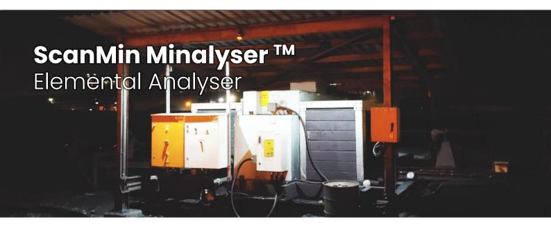
The ScanMin Minalyser™ a Gamma Activation Dual Response Analysis (GADRA) Elemental Analyser. The analyser uses a high- energy Am241Be radionuclide neutron source, which irradiates ALL the material on the belt as result of the temporary excitation of the atoms in the material This provide opportunity to measure two physical reactions:
