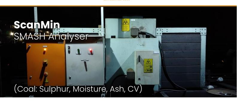
The ScanMin SMASH<sup>™</sup> is a Gamma Activation Dual Response Analysis (GADRA) Elemental Analyser. The analyser uses a high- energy Am24IBe radionuclide neutron source, which irradiates ALL the material on the belt as result of the temporary excitation of the atoms in the material This provide opportunity to measure two physical reactions:
